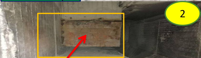
V-sep. inlet impact plate extended for better material flow
